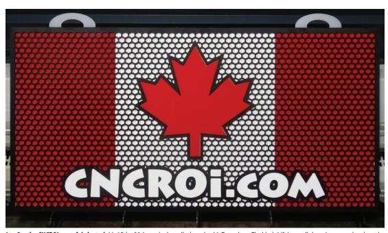
Jon Cantin, CNCROI.com, fabricated this 15-by-30-in. trade show display using his Trotec laser. The black 1/8-in. acrylic layer is mounted to the red and white 1/8-in. acrylic, which is backed up with ¼-in. acrylic. You can watch a video of how he produced it by visiting Jon's blog at www.cncroi.com and scrolling down to "New Acrylic Signage for CNCROL.com". Based in Canada, Jon provides custom CNC laser and router services.
